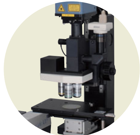
■ レーザ微細加工装置への組込例 Combined with Micromachining Equipment
