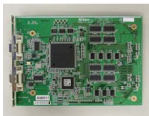
An example of lead-free items: High speed serial interface board employed for the latest IC steppers and scanners
