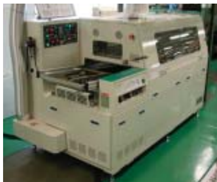
Lead-free flow furnace at Yokohama Plant
