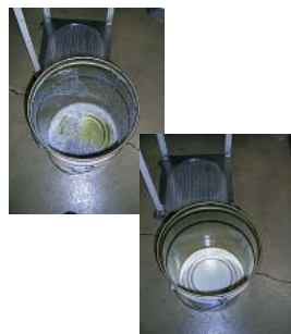
Metal scraps are sucked into the top pail, and cutting fluid into the bottom
