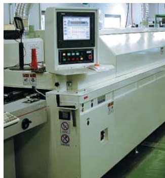
High-performance reflow furnace at Yokohama Plant
