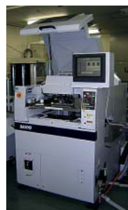
Cream-solder printing machine at Sendai Nikon
